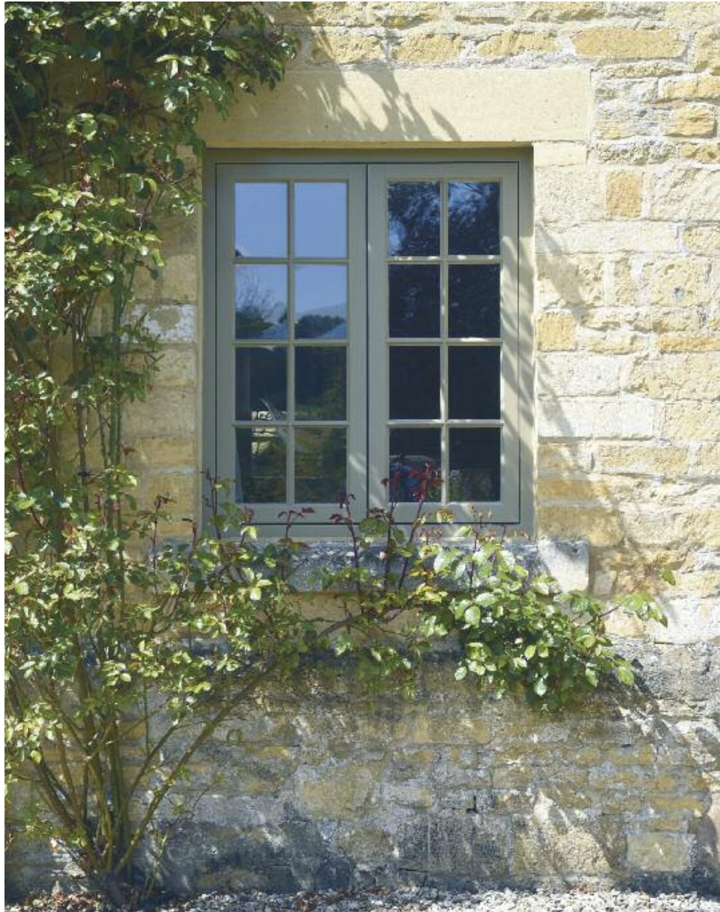
Cottage flush casement windows in the shade of 'Oxide Gold' externally and 'Off-White' internally with 22mm true bars, putty glazed and 14mm ultra slim double glazed units.
